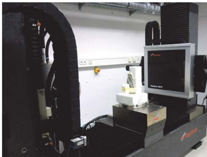
Figure 1: The CT RayScan 250 E device, with a 225 kV micro-focus and with a 450 kV mini-focus X-ray tube and a 2048 × 2048 pixel flat panel detector (cone beam reconstruction) located at the University of Applied Sciences Upper Austria, Wels Campus. Note the fixed limestone sample with the fossil in the centre.
