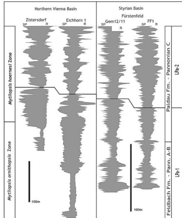
**FIGURE 5:** Geophysical logs (spontaneous potential SP, and resistivity R/Ω) of Lower Pannonian deposits from the Vienna Basin (after Janoschek, 1942, 1943) and the Styrian Basin (after Kosi et al., 2003). Both basins mirror a very similar development which is most obvious in the upper part of the logs (short, funnel-shaped curves). Despite the different tectonic regimes in both basins, and the slight difference in thicknesses of the basin-fills, the overall signature is not fully obscured.
